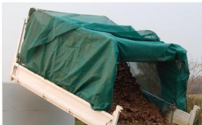
An **optional net kit for the bed** can be added, allowing the waste to be confined in the trailer and thus increasing its loading capacity.
