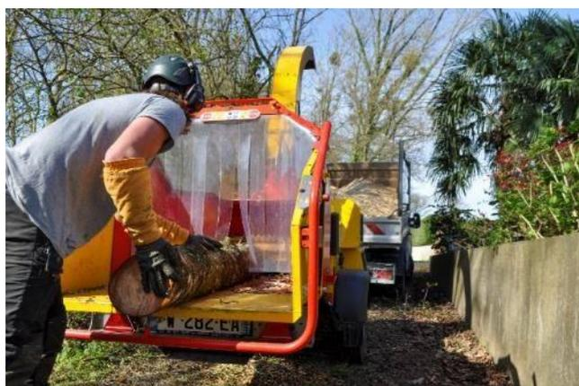
The shredder has a torque reserve to provide extra power when needed, without reducing speed or running the risk of stalling. This is a major advantage when shredding large branches or very hard wood. By adjusting power in this way, the shredder revs up more quickly if the Nostress is triggered.
