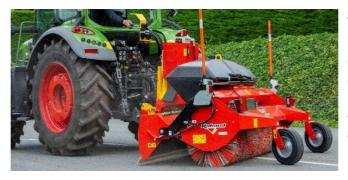
Thanks to its hydraulic cylinder, hopper can be opened easily from the cab via a distributor or radio remote control. The emptying system has been simplified, making it possible to switch quickly from an aligning function to a picking function, increasing its versatility.
