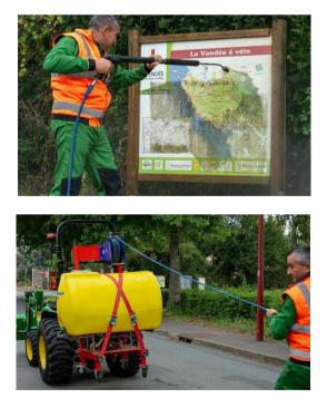
Equipped with a 600-litre water tank, the NHP 600 can work autonomously, even when there's no water nearby. Its **15 I/min high-pressure pump** delivers cleaning power to suit all situations, while guaranteeing low water consumption.
