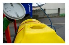
The 600-litre polyethylene water tank is designed to withstand the elements and resist corrosion. Its wide opening makes it easy to fill and maintain.
