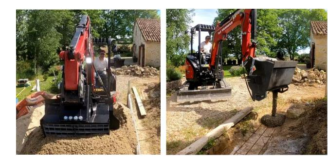
A concrete mixer bucket with blades, specially designed for mini excavators!
