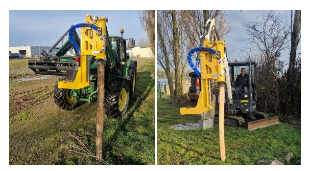
A new hammer for loader and mini excavator post drivers!
