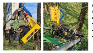
It is easy to adapt to the carrier on any brand of loader, telehandler or mini-excavator thanks to a bolted plate on which **RABAUD can install the quick coupler of your choice**. Also, depending on the hydraulic inlets available on the carrier, RABAUD services can provide a 6-way valve as well as an extension cord.
