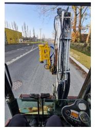
The offset hammer provides excellent **visibility** of the tool from the cab, allowing the pile to be adjusted or straightened as it is driven.
