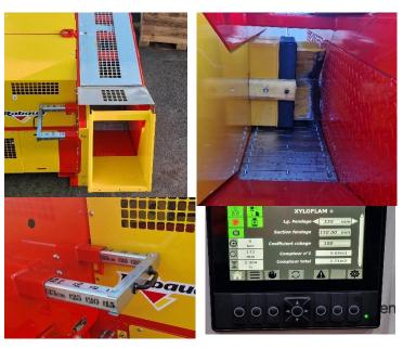
The operation of the XYLOFLAM 330/450+ is simple and efficient: once the timber has been fed into the inlet chute, it descends by gravity onto a metal belt. They are then directed to a splitting cross with a power of 16 tons, which ensures regular splitting, allowing the production of firelighters and logs.
