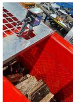
In addition, it is possible to choose for the **XYLOMETER option**, a device that allows the volume of wood produced to be accurately measured, providing additional control over the production process.
