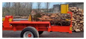
The cylinder stroke is adjustable to reduce the cycle time from wedge release to the start of splitting.
