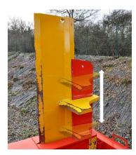
This new model got a new splitting wedge. Its 2 sharp blades, initially arranged in a cross, are now apart from each other. It allows better use of splitting power for optimal results. The wood splits in two on the first edge before being split horizontally on the second.
