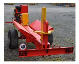
Logs receiving channel has been revised ; **larger, its V-shape centers the log** in relation to the splitting cross, while the Vshaped fins protect the wheels on the road chassis version.
